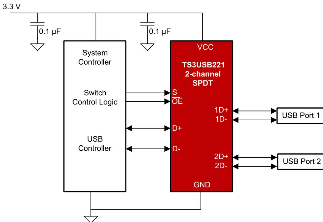
Figure 15. Simplified Schematic
