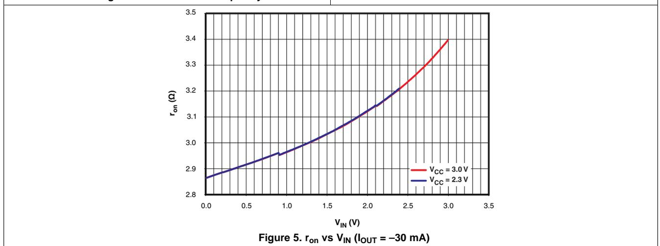
Figure 5.  $r_{on}$  vs  $V_{IN}$  ( $I_{OUT} = -30$  mA)
