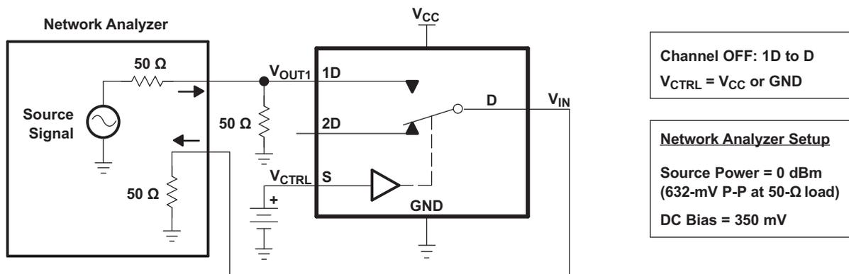
Figure 7. OFF Isolation (O<sub>ISO</sub>)
