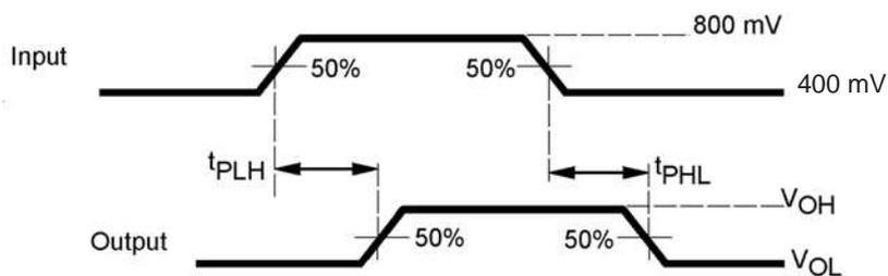
Figure 10. Propagation Delay
