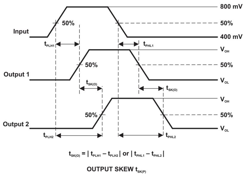
Figure 11. Skew Test
