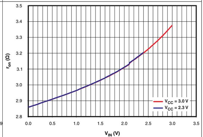
Figure 4.  $r_{on}$  vs  $V_{IN}$  ( $I_{OUT} = -15$  mA)
